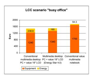
Figure 2: LCC scenario "busy office" for desktop PC and notebooks, prepared using the ENERGY STAR® LCC calculator - http://www.eu-energystar.org/en/en 008b.shtml
